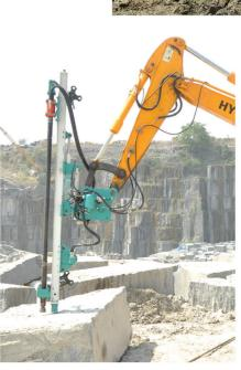
THE DRILL **DESIGN FOR** THE DIMENSION STONE INDUSTRY. IT IS CAPABLE OF DRILLING **VERTICAL AND HORIZONT AL HOLES THAT ENABLE WIRE** CUTTING.
